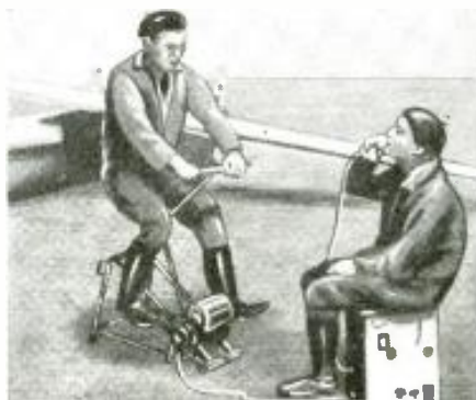
Fig. C The 20-watt transmitter and hand generator which is used for training glider pilots from the ground.
